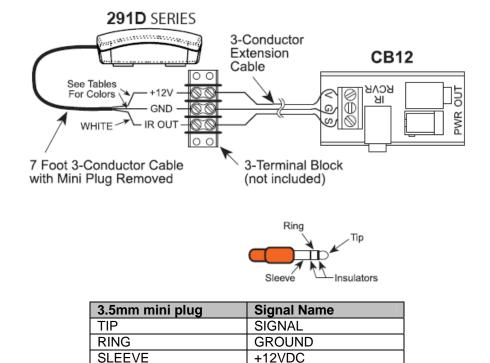
The 3-conductor inter-room cable (24 gauge up to 200', 22 gauge up to 600', 20 gauge up to 2000', 18 gauge up to 5000'), is run to the main room.
