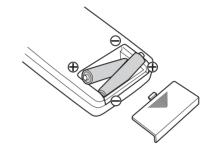
1 Remove the battery compartment cover.
