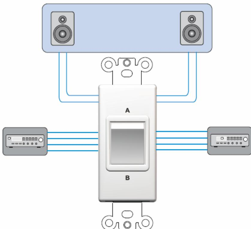
The figure on the left shows the XSSD250W in an application with two sources.
