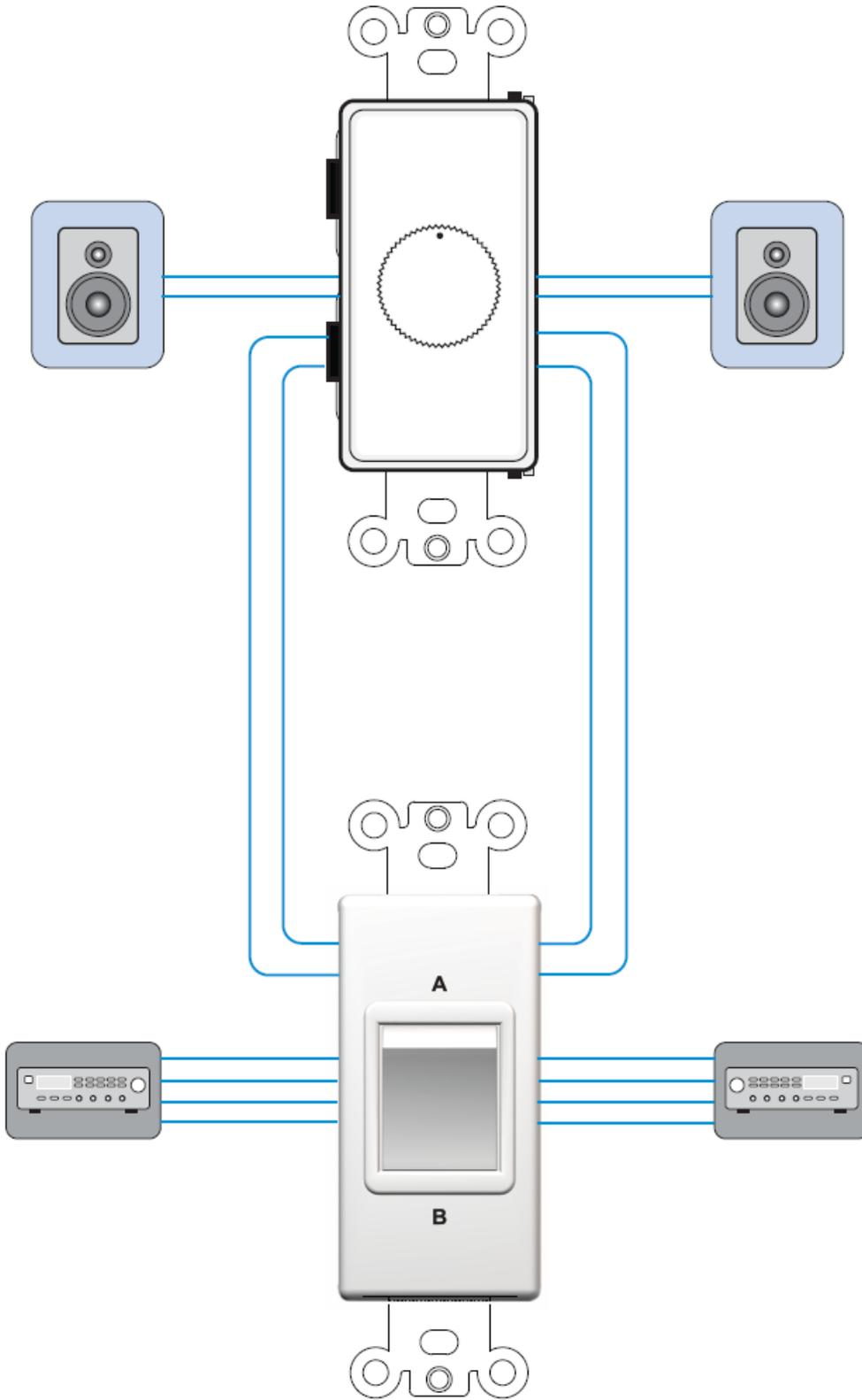
The figure on the left shows the XSSD250W in an application with two sources.
