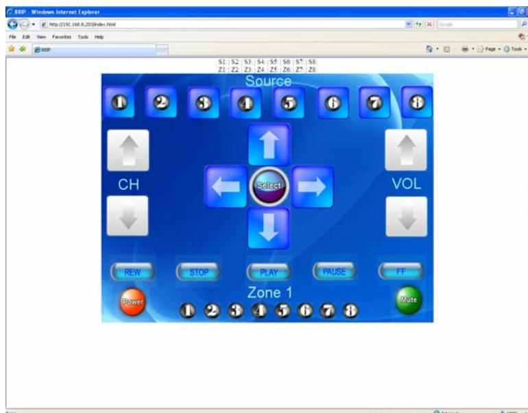
To verify the Ethernet connection, access the MRWC default webpage using a computer connected to the internal network. A web browser, such as Internet Explorer, is required. In the address window, type in the host name <http://mrwc> or the IP address **192.168.0.200**
