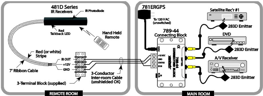
Input connections must be made as illustrated. To extend the emitter wires to a more distant location, you may splice in 2-conductor wire, in the wire gauges mentioned before, as needed.
