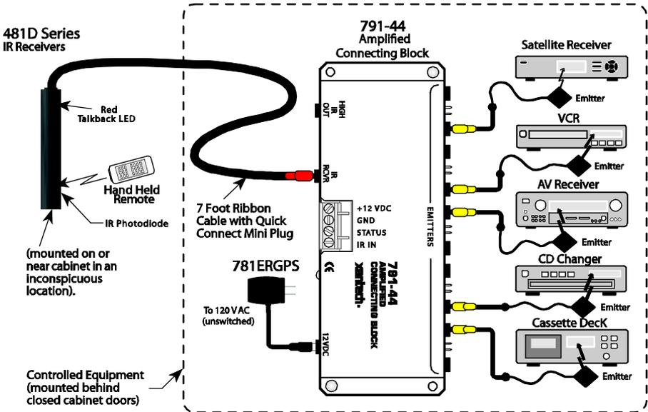
Since the IR receiver is in close proximity to the audio/video equipment, no wiring extension should be required so long as the connecting block is within reach of the 7-foot cable. The 3.5mm stereo type mini plug is connected to the "IR RCVR" jack on the Xantech Connecting Block.
