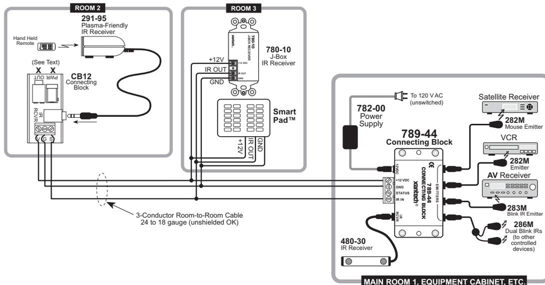
**Figure 3 - Advanced Wiring Configuration using 291-95, CB12, 789-44, 781RG and multiple 286M's**
